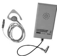
Acoustical pulse detection: A socket on the right side of the Teletector serves to connect either the earphone 6112B-134C or the loudspeaker attachment 6640C. This allows the GM tube pulses to be heard as crackling sounds which makes changes in dose rate easier to recognise.
